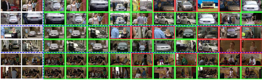
Fig. 3: Comparison of ranked lists on INS2013. Query objects are on the left side. On the right side, the top 10 returns are ranked from left to right: For each example, the upper and lower rows are returned by BL and M6 in Table 1, and the accuracies from top to bottom are 9.46 vs. 25.84, 20.71 vs. 32.37, and 31.21 vs. 65.35. Positive (negative) samples are marked with green (red) bounding boxes. Programme material copyrighted by BBC.
